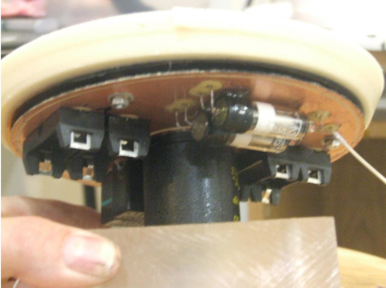
Bottom view of the Static Displacement Field Drive Prototype showing the HV board assembly with electronic tube diodes.
