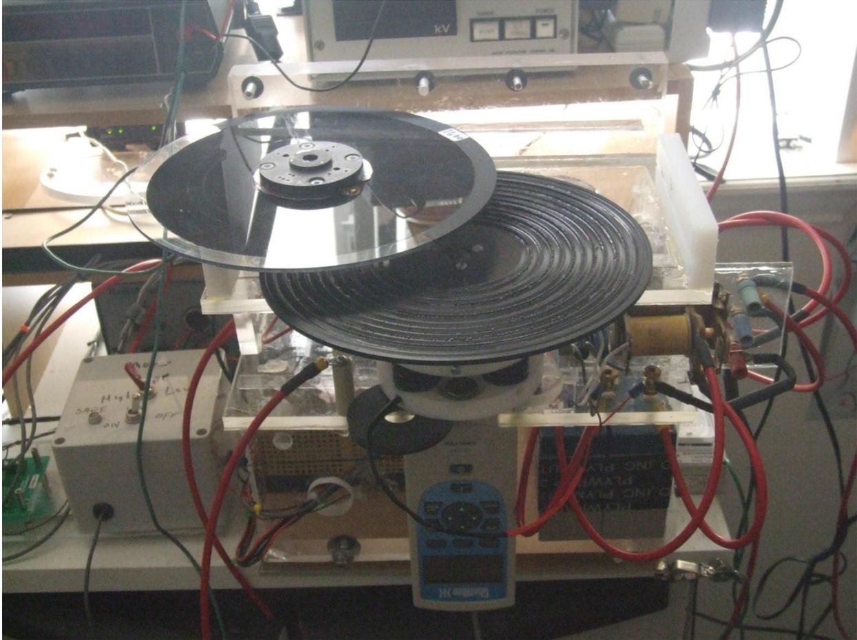
This test fixture is about to be loaded with a dot product disk that generates a radial field when its rotated. The bottom disk is designed to take advantage of the radial electric field that forms from this kind of disk to generate a thrust from. This test fixture is used to test disks from the 9 inch electric field tester to characterize the axial and drag forces from different combinations of disk coatings.
